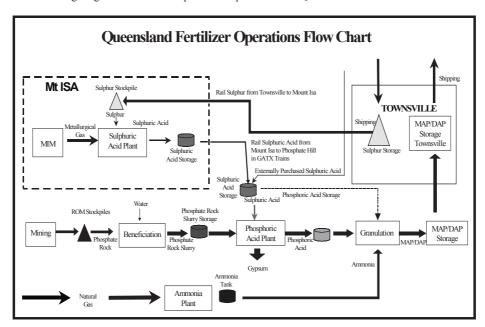
The nameplate capacity of the plant is 975,000 tonnes. Since completion in late 1999, production at the QFO has been steadily increasing. In December 2001, the plant reached an annualised rate of 965,000 tonnes per annum of DAP equivalent. Production in the first half of 2002 has been below capacity largely because of a shortage of sulphuric acid created by operational difficulties at the QFO's sulphuric acid plant and issues with the rail infrastructure between Mount Isa and Phosphate Hill.
